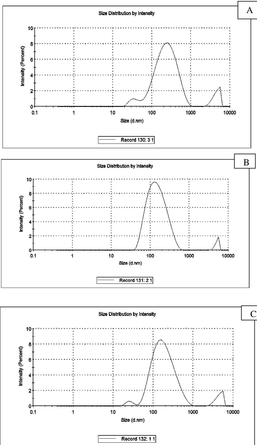
Fig 2: Particle size distribution of 2:8 (A), 3:7 (B) and 4:6 (C) oleic acid emulsion at pH 7
