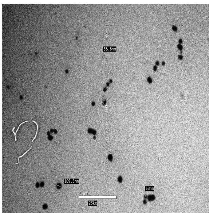
**Fig 1: Electron microscope micrograph of oleic acid emulsion (2:8 oleic: tween 80) at pH 7**
